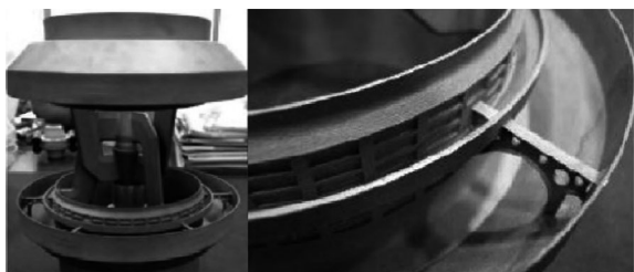
图5 增材制造技术制备RS-25火箭发动机弯曲接头 Fig.5 RS-25 rocket engine bending joint prepared by additive manufacturing technology
