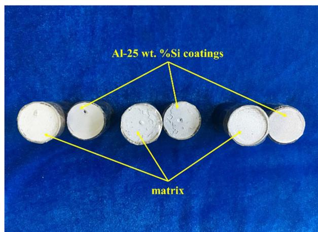
**Fig. 8** Tensile fracture morphology of Al-25 wt% Si coatings samples
